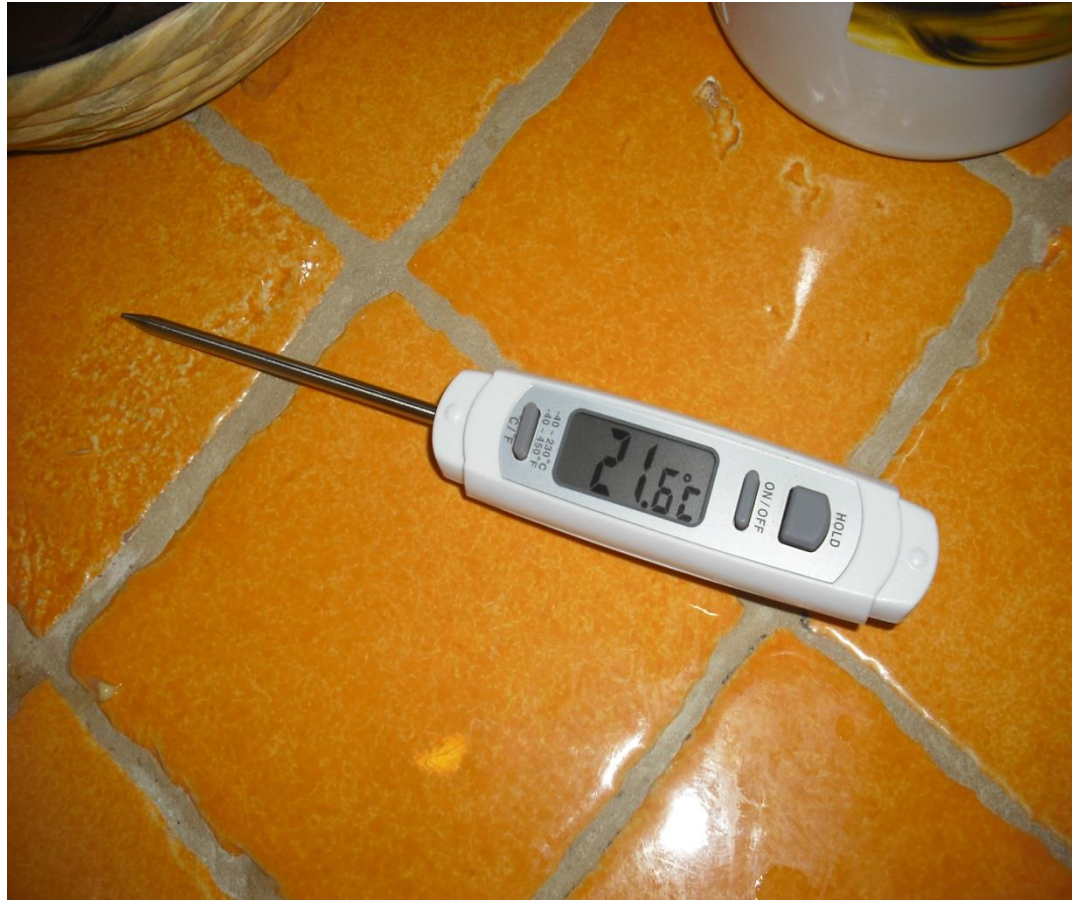
The precision thermometer with external probe
